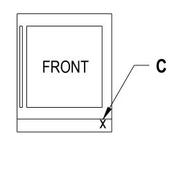
The power cord can be plugged in behind the unit; however for ease of cleaning and service, we recommend the power cord routed to the adjacent cabinet if possible.
